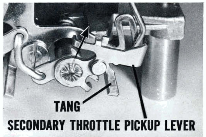
Fig. 4—No secondary operation when choke is on
