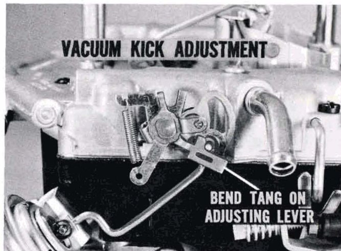
Fig. 25—Tang position determines kick opening
