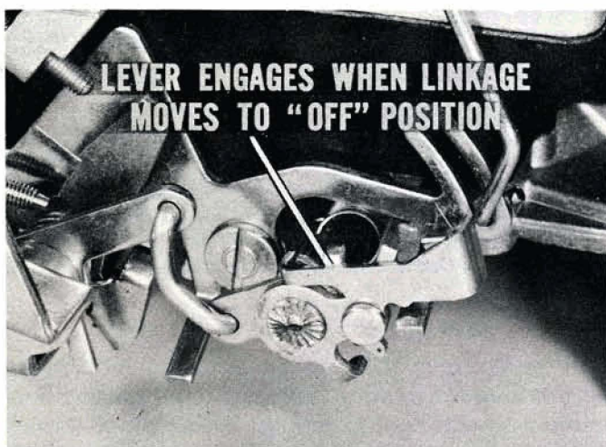
Fig. 5—Lever picks up secondary linkage
